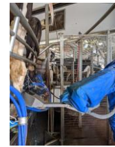
Robotic arm spraying teat dip on cow's udder after milking at Yonkman Dairy
